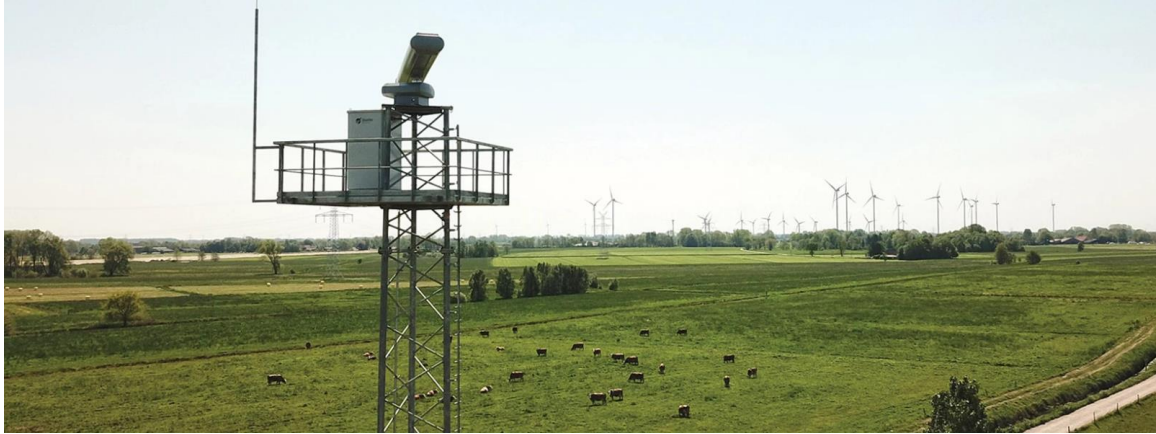
Figure 15 Terma 5002 Radar at a Wind Farm in Germany
