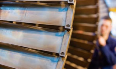
Preparation of last stage LP blades at RWE's Ferrybridge workshops, UK
