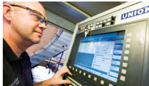
Programming components on CNC Union borer
