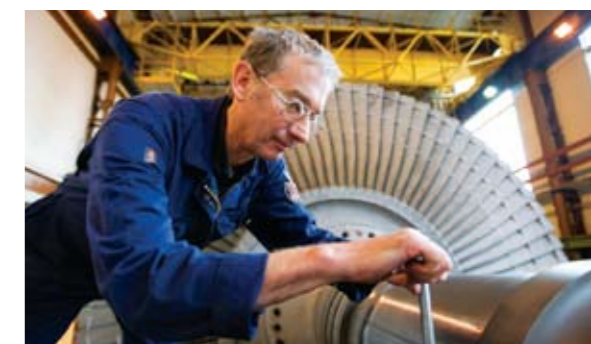
Commencement of machining work on LP rotor
