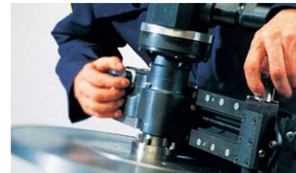
On-site machining of a flange face
