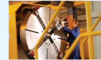
Chuck setting on CNC lathe
