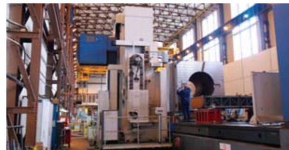
Machining a 90 tonne component on the CNC Union Borer
