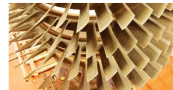
Gersteinwerk destack Top: GT compressor rotor blading
