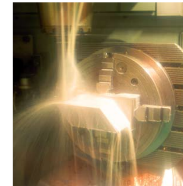
Compressor diaphragm manufacture utilising multi axis CNC machining
