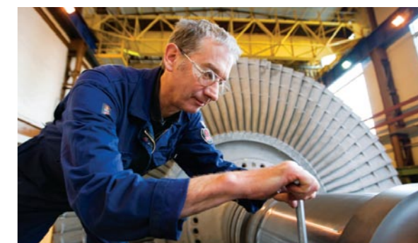
Commencement of machining work on LP rotor
