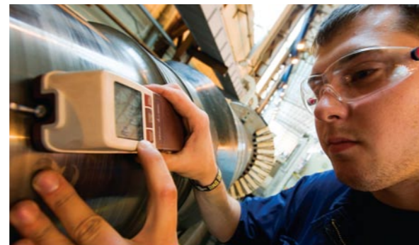
Carrying out a surface finish assessment
