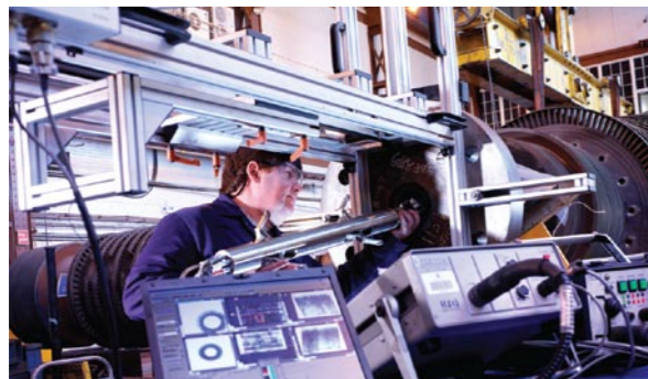
Automated rotor bore inspection using array Eddy Current and UT imaging technology
