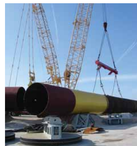
Monopiles like this one are the mainstay of each wind turbine.
