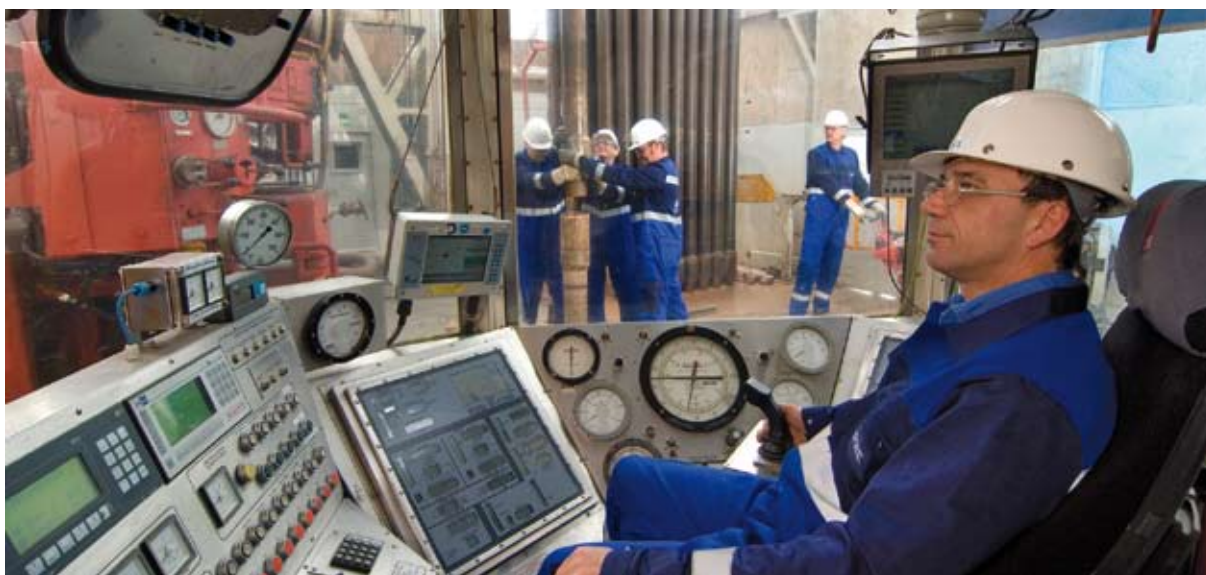
In the control centre of the T-160 drilling rig: remote directional control guides the drill bit into the reservoir with great accuracy.
