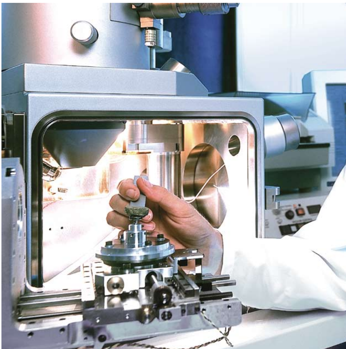
A sample is prepared for analysis under the scanning electron microscope in the RWE Dea laboratory.
