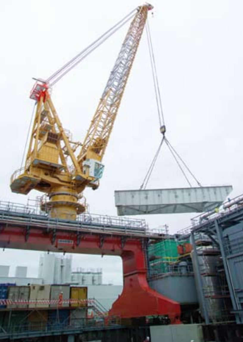
By the end of 2005, much of the equipment and facilities on Mittelplate Island had been upgraded, optimised or replaced. This also includes a new, high-performance portal crane with a slewing range that is adequate to meet all lifting requirements on the entire island.
