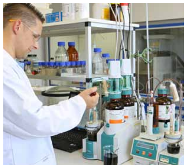
The water content in crude oil is determined by the RWE Dea laboratory with the aid of the Karl-Fischer titrator.
