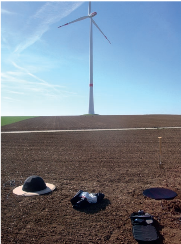
Figure 4.5-1 (right): Measurement points MP2 and MP3 at a distance of 300 m from the tower axis. Reverberant plate and double wind screen (left), spanned hole in the ground (right). Photo: Wölfel company
