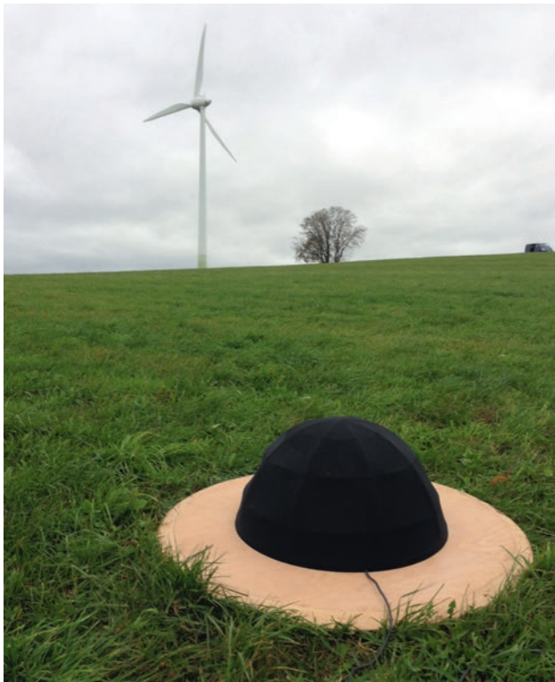
Figure 4.3-1: Measurement point MP1 with microphone, reverberant plate and dual wind screen. In the background: wind turbine WT 2 at a distance of 120 m. Photo: Wölfel company.
