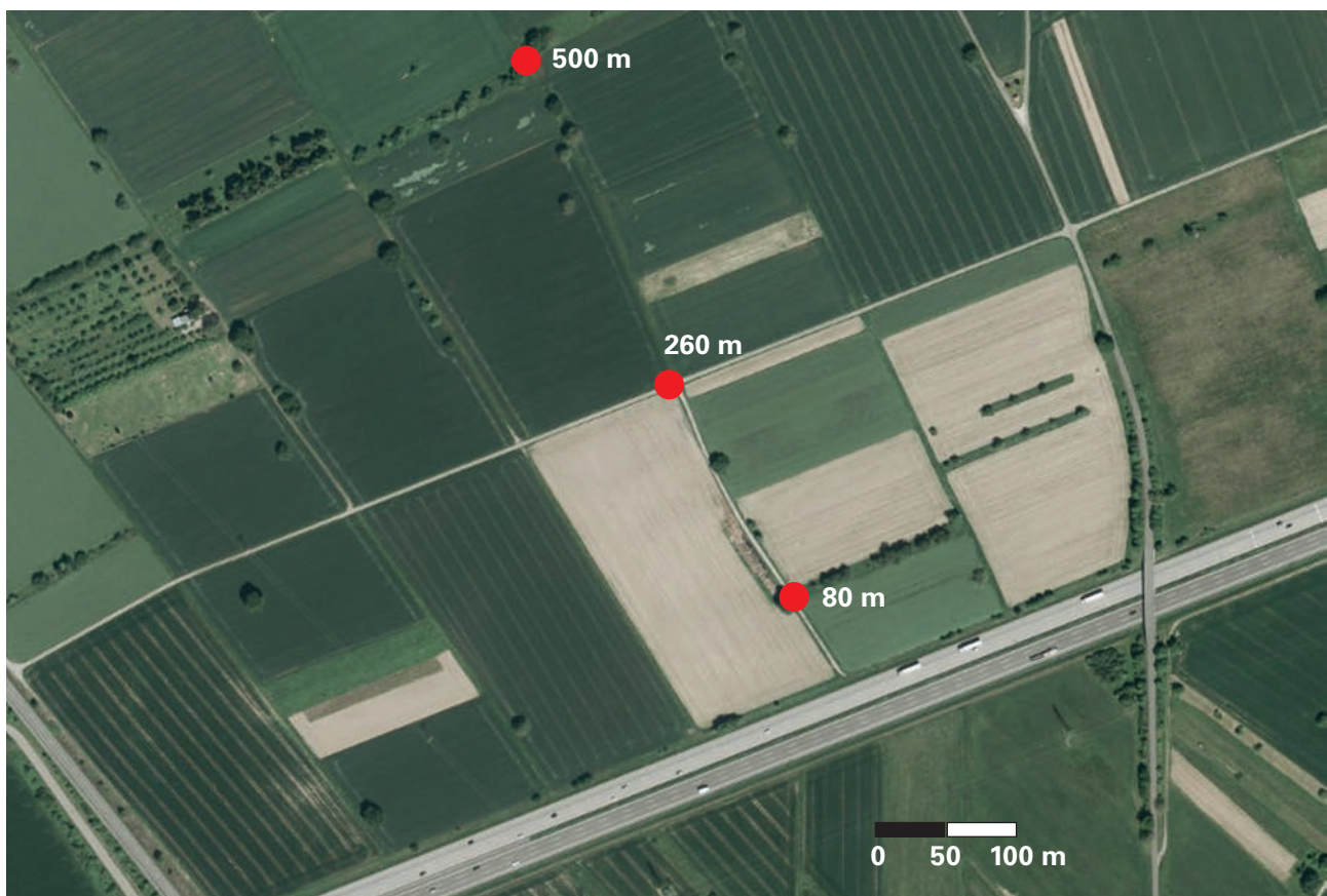
Figure 5.3-1: Location of the measurement points at the A5 motorway south of Karlsruhe near Malsch, indicating the distances between the microphone positions and the centre of the motorway. The town of Malsch is located outside of the picture at the bottom left. The B3 main road is located above the picture. Picture source: LUBW, LGL
