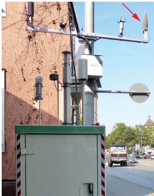
Figure 5.2-2: LUBW measuring station for detecting road traffic noise in Reutlingen, Lederstrasse. The arrow shows the location of the microphone. Photo: LUBW
