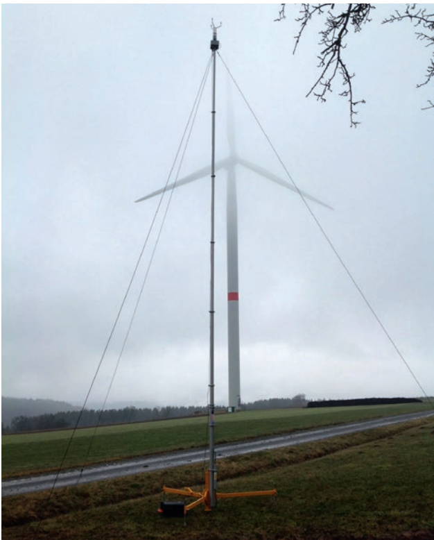
Figure 4.2-1: Wind measurement mast with view in direction of the wind power plant being measured. Photo: Wölfel company
