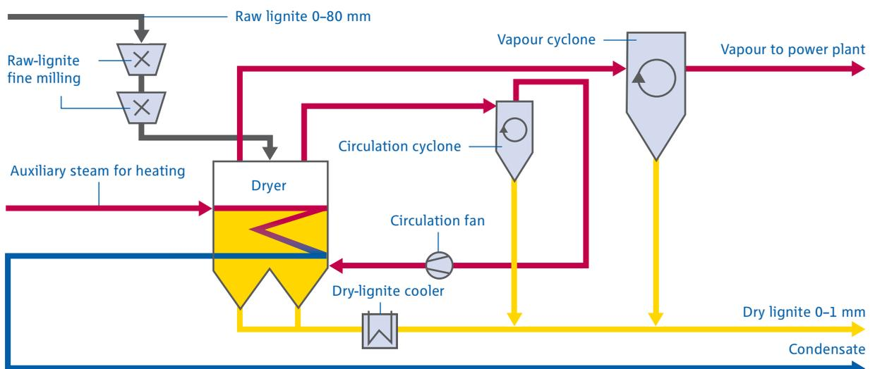
Process principle: WTA as low-cost variant
