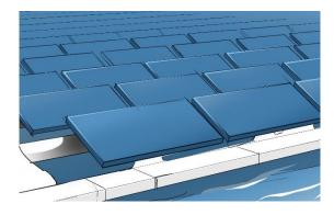
Example of a possible system design for floating PV. In the »PV2Float« project, several different designs and substructures are implemented on an open pit lake.
